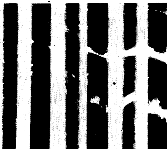
Figure 3. Effect of cycling the temperature between 300 and 77 K on a glass tube containing apiezon N grease under an atmosphere of helium gas. Beginning on the left, the first, third, and fifth photographs were taken with the tube at 77 K. The second, fourth, and sixth pictures were obtained after the grease temperature returned to 300 K
